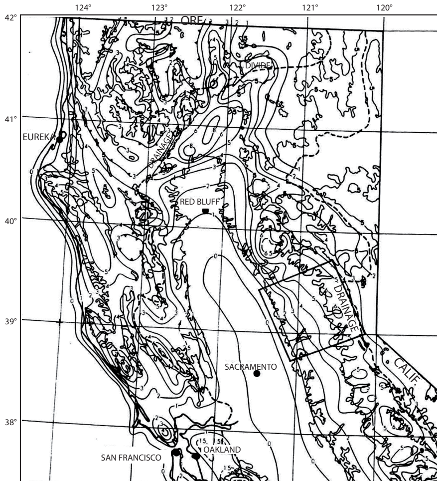
Figure 3.9. Six-hour orographic PMP (inches) for January (square delineates Blue Canyon orographic model test area; United States Weather Bureau, 1961a)
